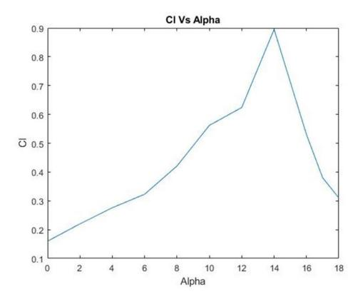
Fig 6: CL vs alpha graphs obtained by simulations in ANSYS
