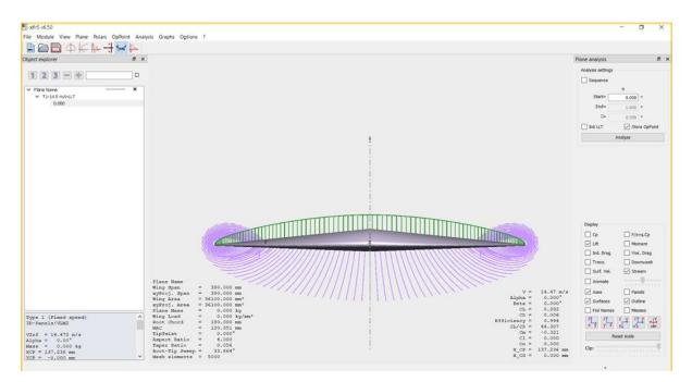
Fig 2: the streamlines flow simulation over delta wings in XFLR5
