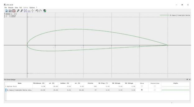
Fig 1: NACA 4415 air foil using for delta wing design in XFLR5 software
