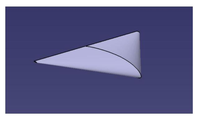
Fig 3: the computer aided designed delta wing using NACA 4415 in CATIA
