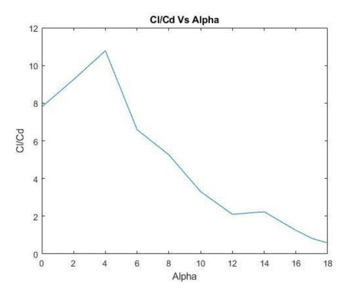
Fig 7: Cl/Cd vs alpha graphs obtained by simulations in ANSYS
