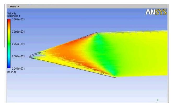
Fig 8: This is a streamline flow simulated in ANSYS for Delta wing
