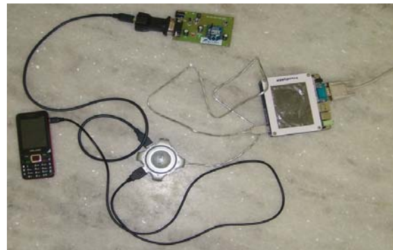
Fig :5- Interfacing of the GSM AND MPMS Module
