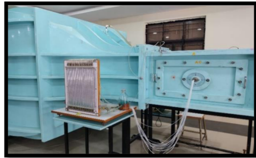
Fig 1.2. Pressure probes connected to the multitube manometer
