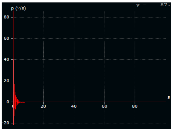
Fig 9. Roll rate deviation P = d\theta/dt , Response to disturbance ( P(°/s) vs T(sec) ).
