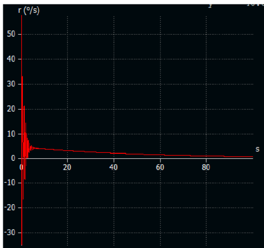
Fig 10. Yaw rate variation r = d\psi/dt , Response to disturbance ( r(°/s) vs T(sec) ).
