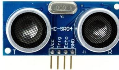
Gambar 2.4 Modul sensor jarak ultrasonik HC-SR04 (Sakti, 2015)
