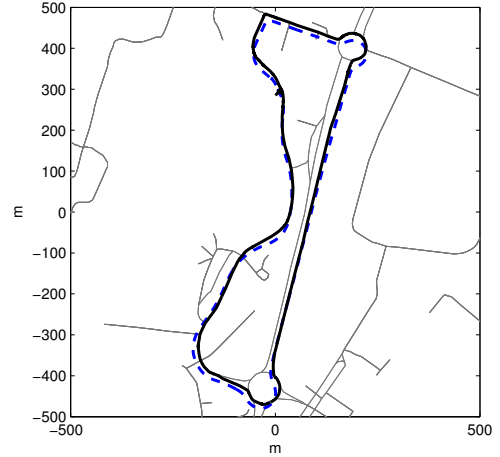
Figure 2: Trajectory -dashed- vs. map-matched trajectory -plain- in an ENU frame centered on the map.
