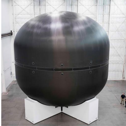
Figure 1: SpaceX liquid oxygen fuel tank prototype for manned Mars missions aboard the Interplanetary Transport System [4]
