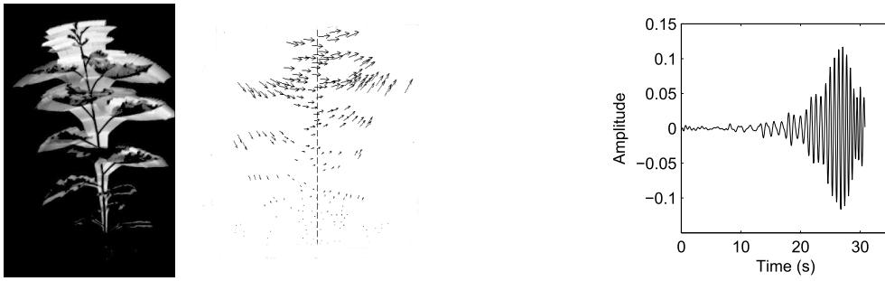
Figure 2. Left: Visualization of the oscillating motion using image superposition. Center and right: Example of the result of a BOD decomposition. Dominant spatial structure, or chronos (center), and the corresponding temporal structure, or topos (right). The peak of the chronos corresponds to a resonance and allows the identification of the modal frequency.
