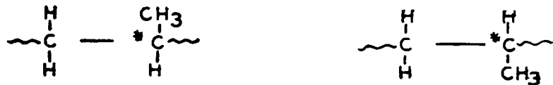
TWO CONFIGURATIONS OF ASYMMETRIC CARBON ATOM OF THE MONOMER UNIT OF POLYPROPYLENE.
