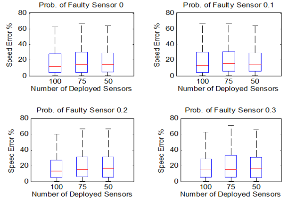
Figure 5. Experiment 1 results. Distribution of the speed error under different scenarios. Each panel corresponds to a different probability of faulty sensors.
