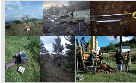
Figure 2 – Example of field investigation (DGPS monitoring, peat extraction for C14 datation, geophysics, Pressler extraction on a tree, borehole)
