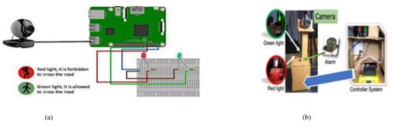
Figure 4. The implementation of the pelican crossing system for predicting the pedestrian age, (a) Schematic, (b) Our Prototype
