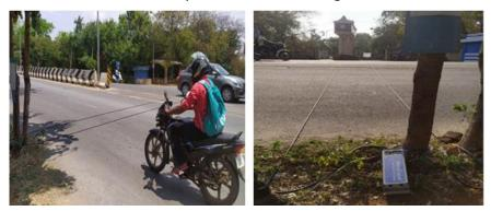
Fig. 2. Installed MetroCount unit for the Traffic study
