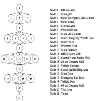
Figure 4. Directed-graph based on The Adversary Sequence Diagram (ASD).
