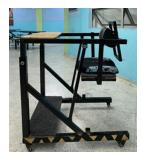
Figure 1. Transfer Lifter Assistor
