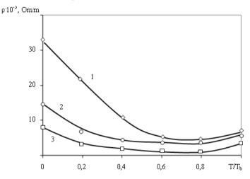
Fig. 1. Influence of the baking temperature of the carbide powder on the electrical resistivity: 1 - TN20; 2 - T14K8; 3 - VK8
