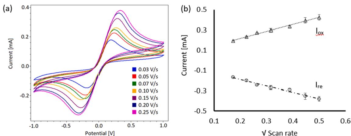
Fig. 1. Electrochemical characterization of the paper-sensor. (a) Cyclic voltammograms with increasing scan rates measuring  $2.5 \text{ mM}$  ferri/ferrocyanide. (b) The extracted peak current values as function of the square root of the scan rates.
