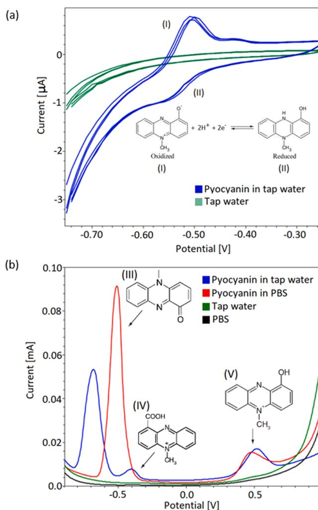
Fig. 2. Electrochemical fingerprint of pyocyanin in water. (a) Cyclic voltammograms of  $5 \mu\text{M}$  pyocyanin in tap water measured with the paper-based sensors. (b) Square wave voltammograms of tap water and PBS spiked with  $200 \mu\text{M}$  pyocyanin vs the backgrounds.
