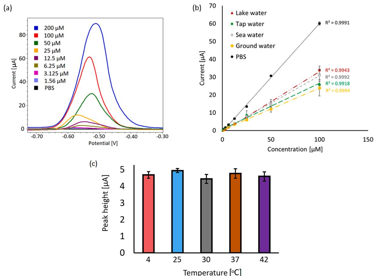
**Fig. 3.** Quantification of pyocyanin in water. (a) Square wave voltammograms of increasing concentrations of pyocyanin spiked in PBS. (b) Standard curves of pyocyanin in PBS, lake water, tap water, sea water and ground water. (c) Temperature effect on peak height. The extracted peak heights belonging to a constant pyocyanin concentration spiked in tap water and measured at different temperatures.
