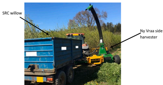
Fig. 4. Ny Vraa side harvester attached to tractor and trailer, in use at AFBI Large Park Hillsborough, Northern Ireland. Photo taken by Oliver Carville. SRC = short rotation coppice, AFBI = Agri-Food and Biosciences Institute.
