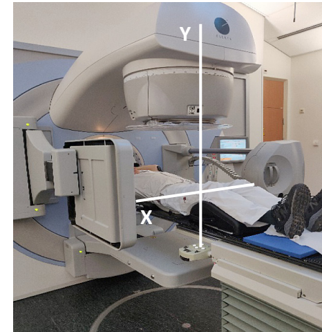
Figure 4. Image of a linear accelerator (Elekta) with on the vertical axis (Y) on the top the MV source and on the bottom the MV imager panel, on the horizontal axis (X) on the right the kV source and on the left the kV imager panel.
