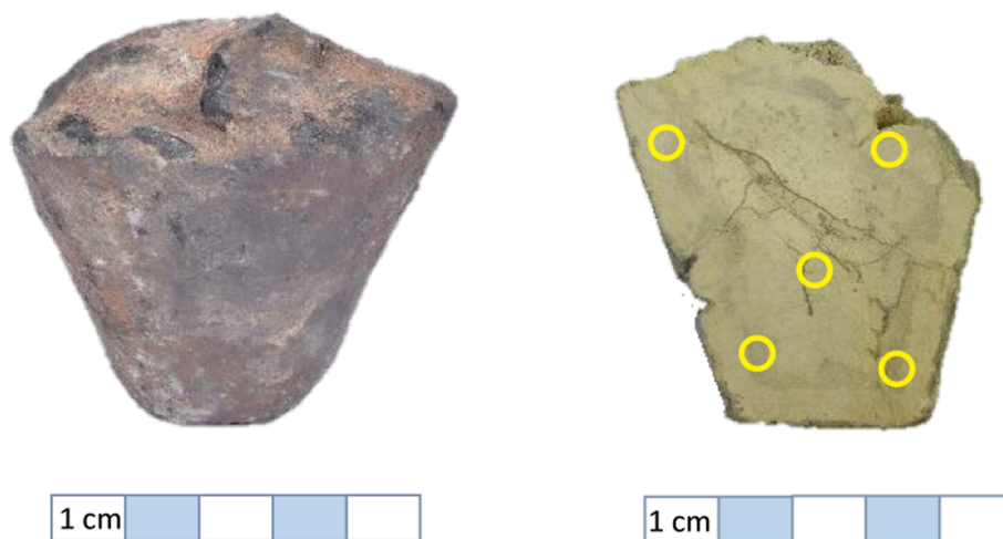
Fig. 1. Left, exterior view of a Venetian lead white cone and right interior view of a cone that was cut in half. Note galena-rich rim. Yellow dots mark sampling locations. Approximate cones size: width, 5 cm at the bottom 8 cm at the top; height 7–10 cm; weight circa 500 gram.
