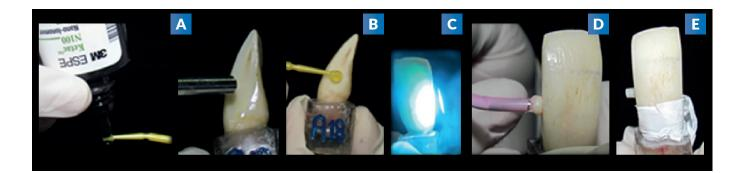
A: Application of the Ketac Nano primer. B: Air blowing the Ketac Nano primer. C: Light Curing the Ketac Nano primer. D: Application of the nano-filled resin-modified glass ionomer cement Ketac N 100 on the dentin surface. E: Specimen with the restoration completed on the right side.
