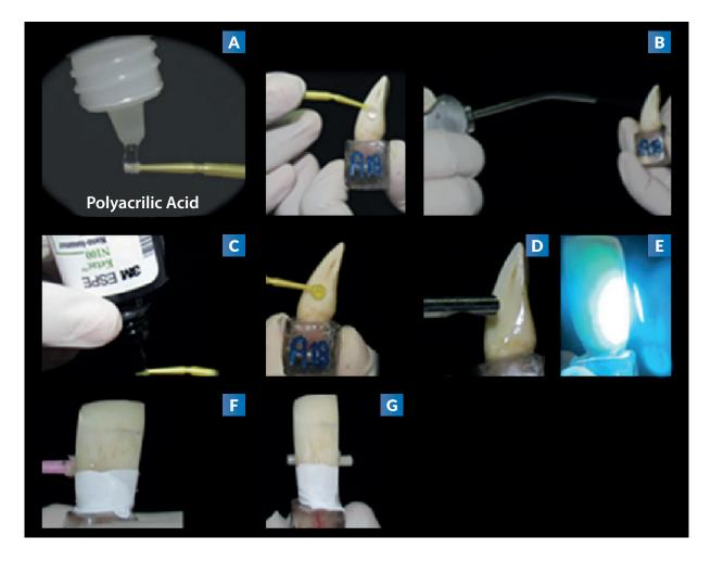
A: Dentin conditioning with polyacrylic acid. B: Washed the Polyacrilic acid an dried of the dentin surface. C: Application of the Ketac Nano Primer. D: Air blowing the Ketac Nano primer. E: Light Curing the Ketac Nano Primer. F: Application of the nano-filled resin-modified glass ionomer cement Ketac N 100 on the dentin surface. G: Specimen with the restoration completed on the left side.
