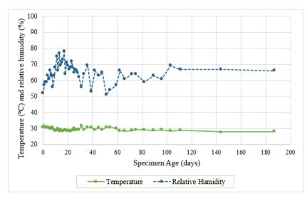
Fig. 3 - Temperature and relative humidity under the tropical indoor condition
