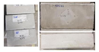
Fig. 1 - locations of strain discs on the specimen
