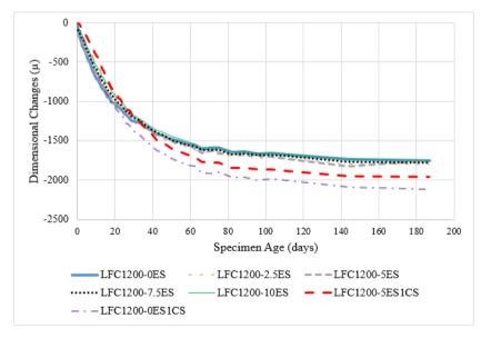
Fig. 2 - Dimensional change of the LFC under the tropical indoor condition
