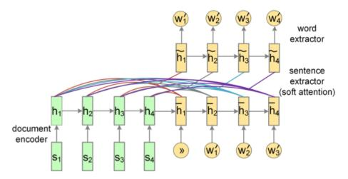
Figure 6: Attentional Encoder-Decoder Architecture, Neural Summarization by Extracting Sentences and Words
