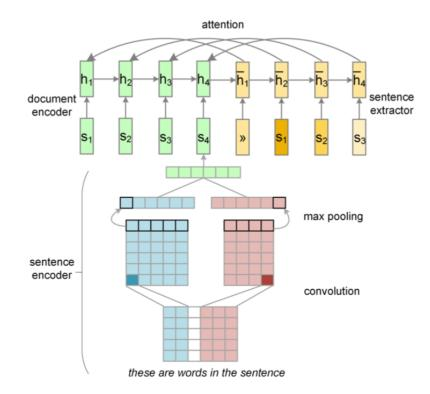
Figure 5: Attentional Encoder-Decoder Architecture, CNN + RNN
