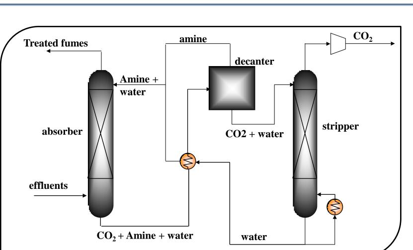
Aqueous solutions of amines are selective carbon dioxide ( $CO_2$ ) absorbents [1,2]. They are used in CO<sub>2</sub> capture processes working on absorption/desorption cycles.
