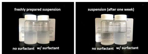
Figure 5. Spray suspensions at the start (a) and after a week (b) of observation. The silane-functionalized silica suspension was more stable with HTAB addition.
