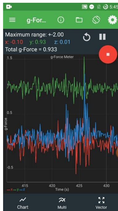
Figure 8. A spike in the G-force (blue) due to hard braking
