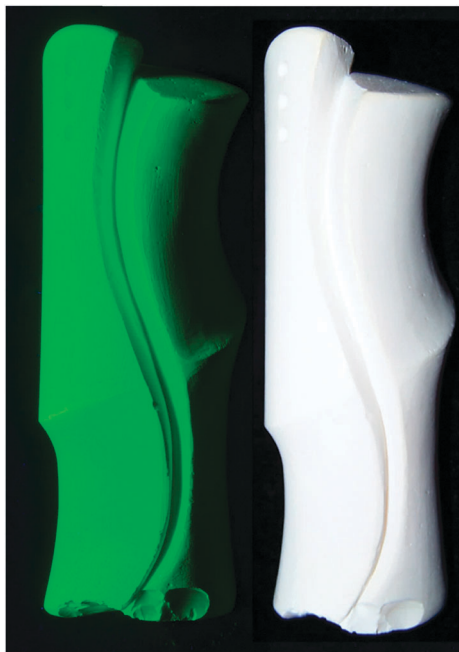
Fig. 6 Photograph of the sculpted piece of the MSM–YAG:Tb composite with a width/height dimension of 30/100 mm before (right) and after (left) 375 nm excitation.
