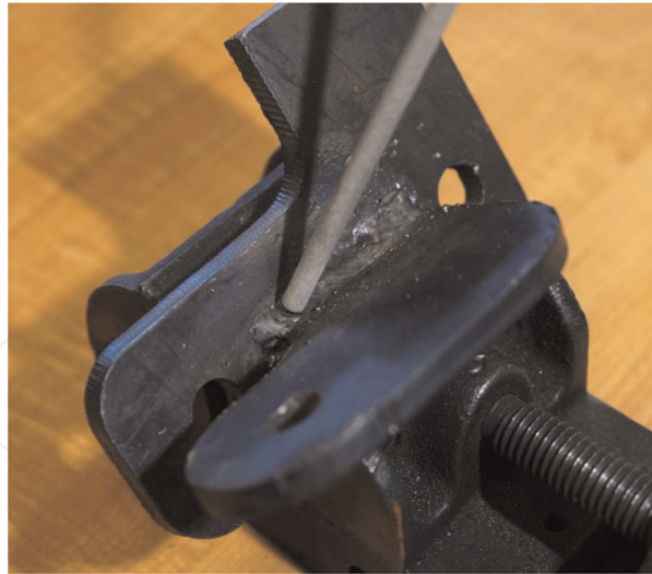
Figure 6. Base material orientation and working position for flat position fillet weld (1F).
