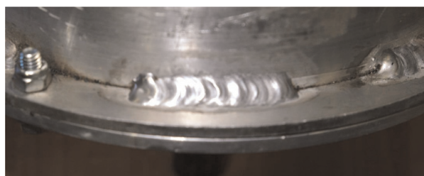
Figure 5. GTAW/TIG fillet weld on aluminum material.
