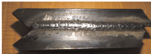
Figure 21. A fine cap fillet pass used to finish joining two separated pieces, which may be ground flush for a solid appearance.
