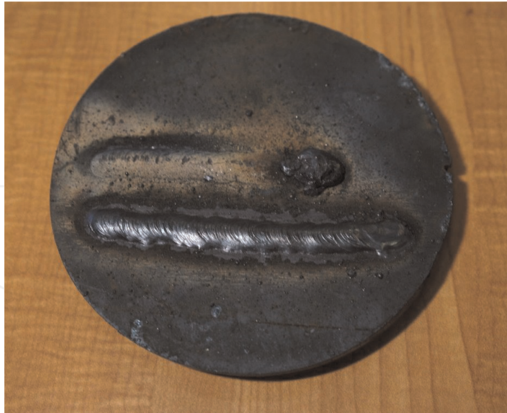
Figure 2. Stick welded components showing the splatter from the process.
