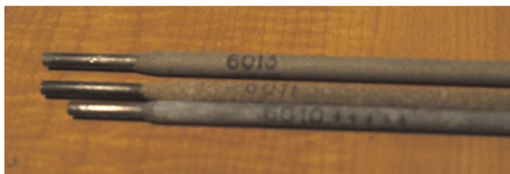
Figure 1. Electrode specification stamped on the flux coating of a typical welding rod.
