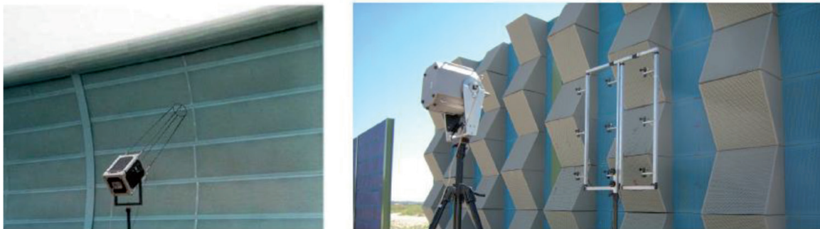
Figure 2. Measurement according to the “Adrienne” method (left) [30] and “QUIESST” method (right) [31].
