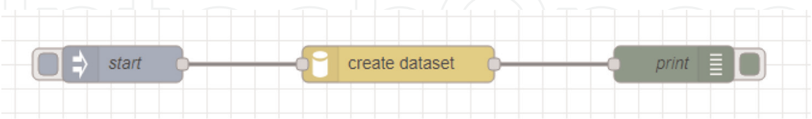
Figure 2. Flow for loading a csv file, shuffling it, and creating a training and a test partition.
