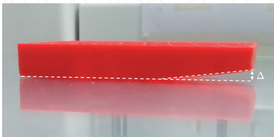
Figure 2. Warping of a cuboid print model.
