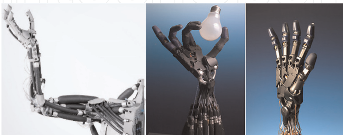
Figure 3. The bionic musculoskeletal robots of the FESTO Airic's arm and the SHADOW hand [5, 6].
