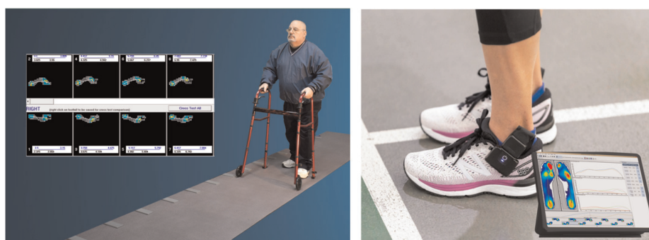
Figure 5. Pressure-based systems to analyze gait and posture. From left to right: GAITRite and Xsensor. Images obtained from the official website of Xsensor [58] and GAITRite [59].
