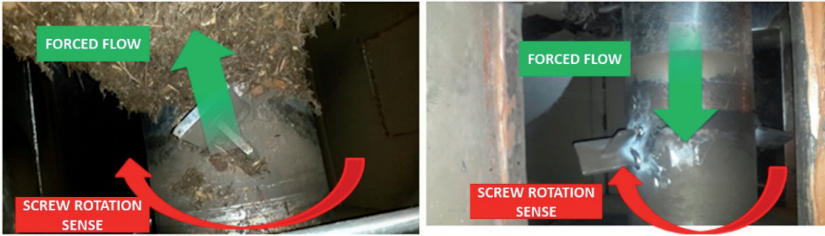
Figure 7. Thread shaft fin position before (left) and after (right).
