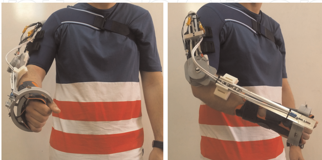
Figure 3. Elbow exoskeleton over the human body.
