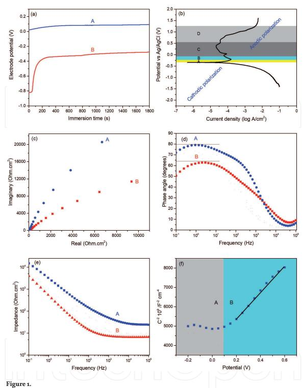
Illustration of the corrosion properties of metallic materials; (a) open circuit potential (OCP), (b) potentiodynamic polarization, (c) Nyquist plot, (d) Bode phase angle plot, (e) Bode impedance plot, and (f) Mott-Schottky plot.
