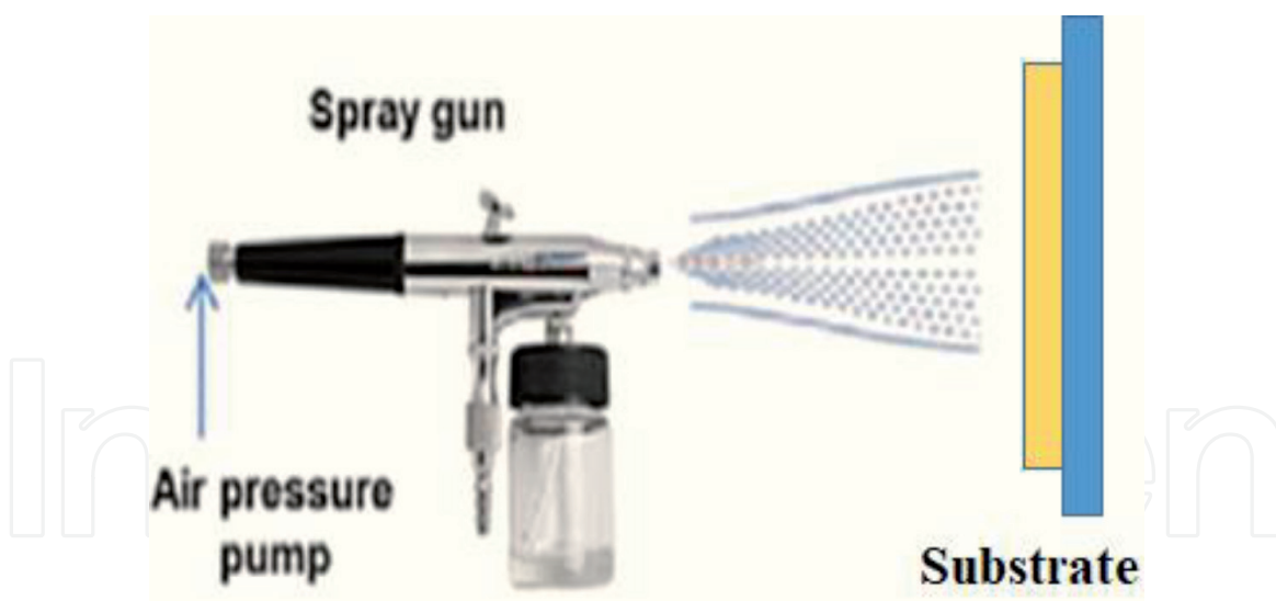
Figure 12. Schematic of the spin-spraying method.
