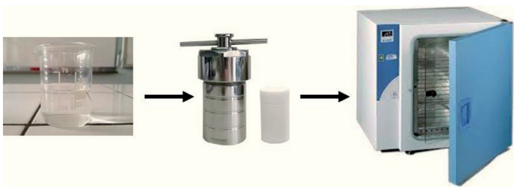
Figure 11. Schematic of the hydrothermal method.
