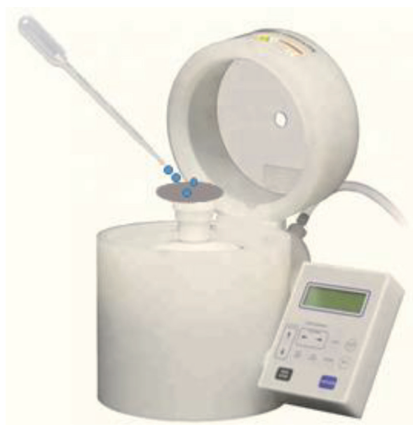
Figure 13. Schematic of the spin-coating method.
