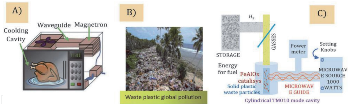
Figure 2. Microwave heating. (A) A typical 1000 Watts, 2.45-GHz domestic microwave oven (MWO) cooking a chicken. (B) Plastic pollution derived from tons and tons of waste plastic bottles and supermarket bags. (C) Clean production of H_2 by microwaving waste plastic bags and bottles mixed 1:1 with the catalyst FeAlO_x within a cylindrical cavity, the input power is 1000 Watts, and H_2 gas is liberated and carried toward a separate container. The cylindrical cavity operates in the TM_{010} mode.
