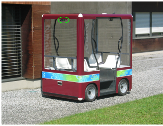
Fig. 9. VipaLAB: electrical vehicle used in the experiments here. It is equipped with a Marlin F-1318 camera (circled in green) and an odometer.
