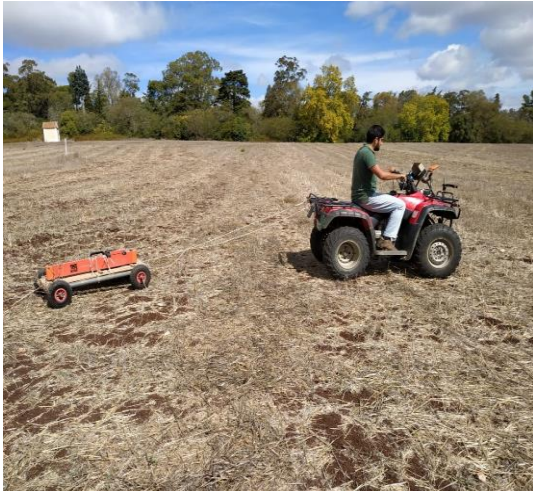
Figure 9- Electromagnetic induction ECa measuring method. Source: Own source
