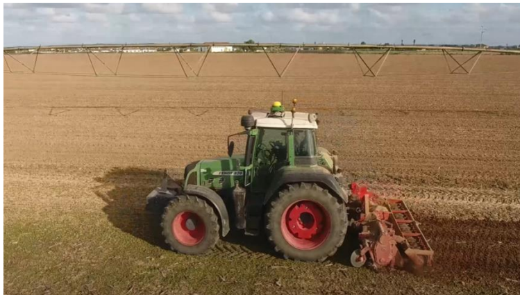
Figure 18- Tractor with a built-in GPS RTK and a power harrow. Source: Adapted from Milho Amarelo.
