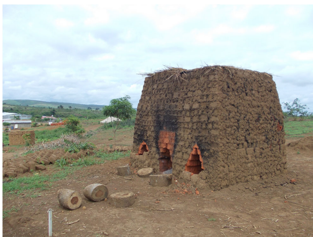
Fig. 4 Medium size mud brick oven and some fuelwood
