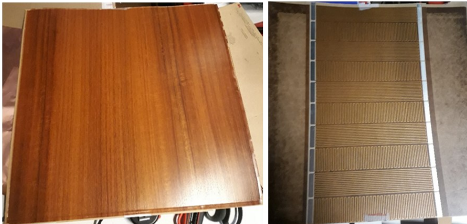
Figure 1. 50 x 50 cm sample of ten high pressure laminated resistance patterns with resistance of 4.5 \Omega each.
