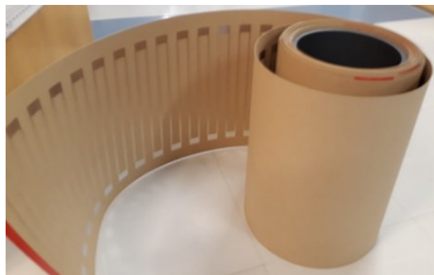
Figure 6. Aluminium heating pattern with kraft paper substrate.
