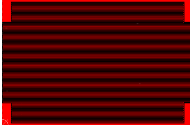
Figure 20. Third version – single layer, connections in one direction.
