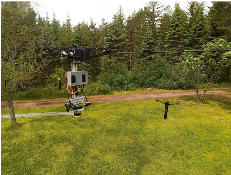
Figure 32. Testing and filming setup including the cable drone and a Wiral LITE.
