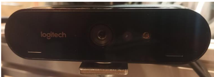
Figure 24. Logitech BRIO 4K attached to the portable sensor system.
