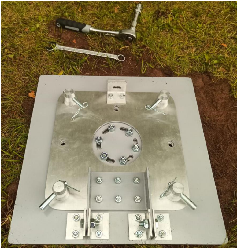
Figure 14. Assembled ground base with assembly tools.
