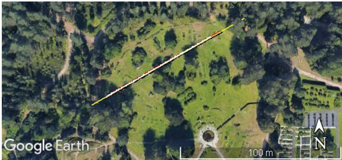
Figure 37. Position data from initial tests' first (black), second (red), and third (white) manual test run collected with Xsens and plotted into Google Earth while yellow line represents the cable.
