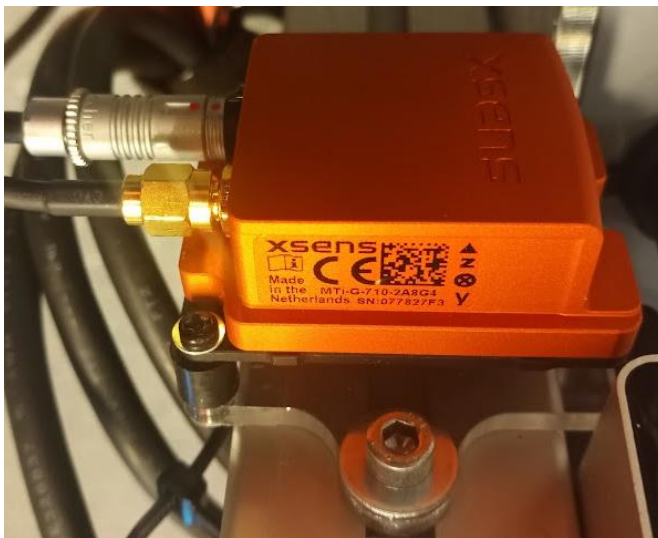
Figure 25. Xsens MTi-G-710 GNSS/INS attached to the portable sensor system with dampeners.
