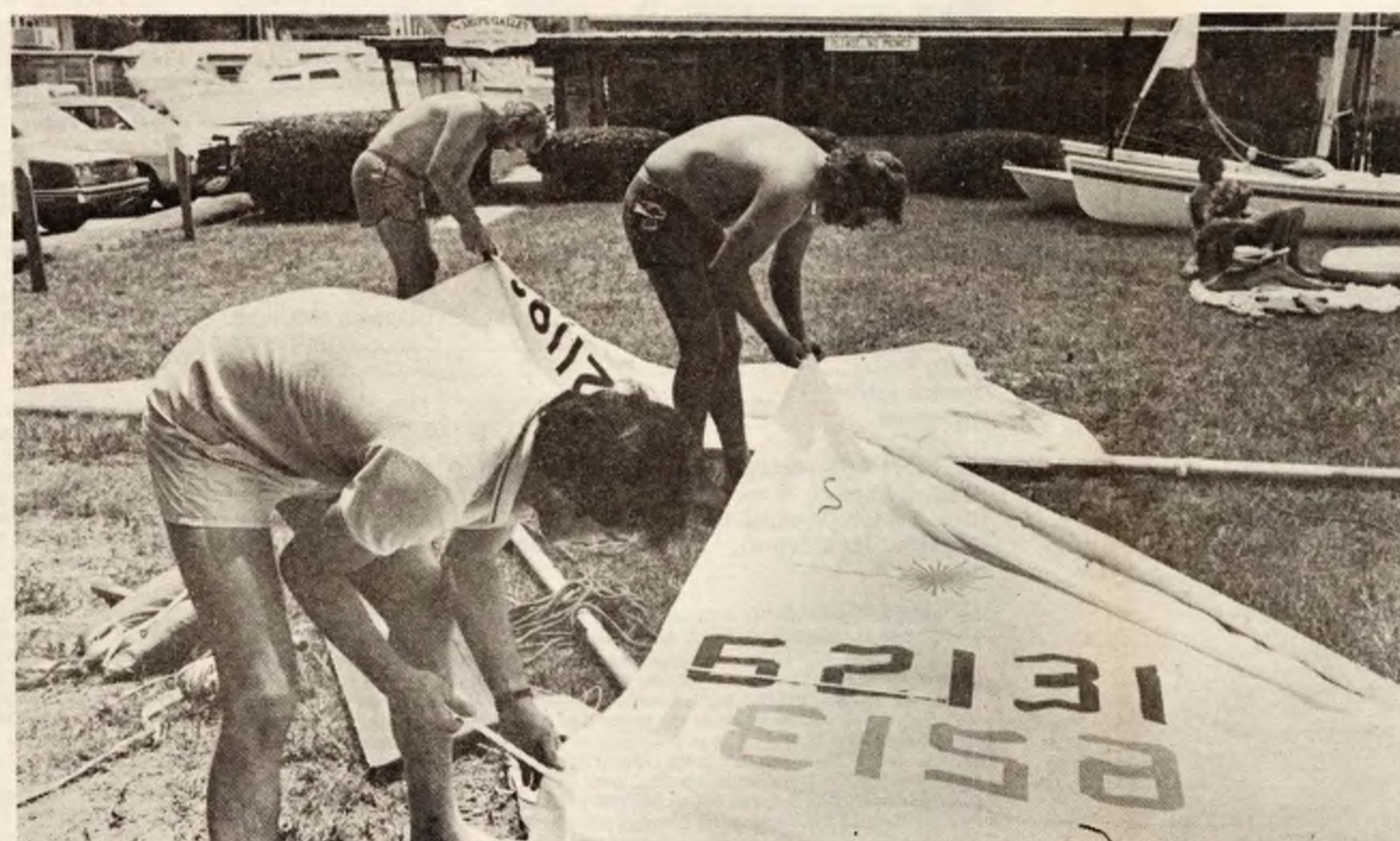
After the sail is in position on the mast, Miles and Courtland slip the battens (stiffening rods) into the sail.
