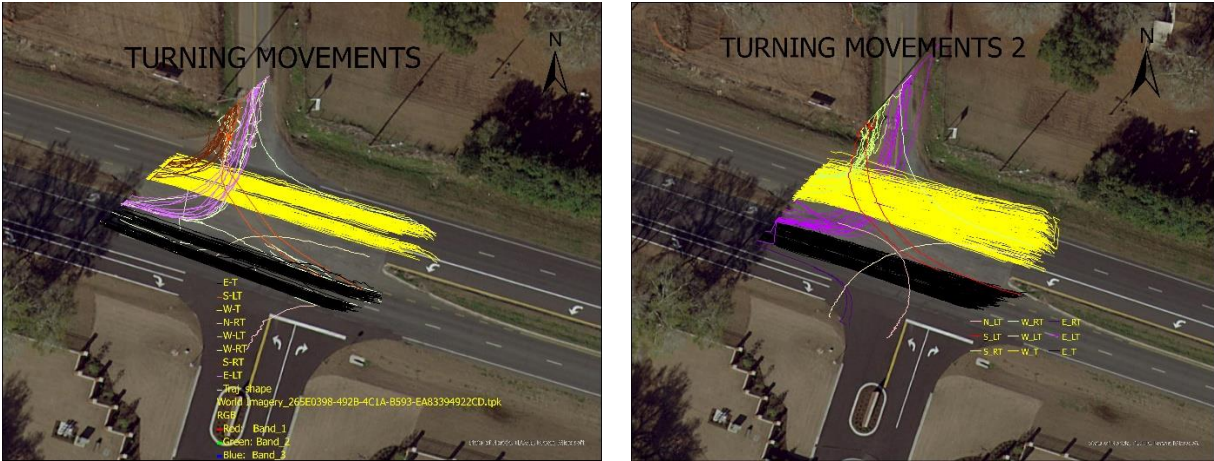
Figure 5-3: Vehicle's trajectory lines categorized by their turning movements for the first and second drone footages
