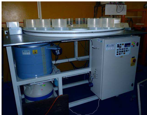
Fig. 3: Radiometry apparatus with a 70-80 % efficiency Ge detector.
