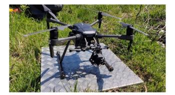
**Figure 4.** The specifications of the UAV DJI Matrice 210 V2, equipped with the Zenmuse XT2 dual sensor, make it suitable for this kind of prospecting.
