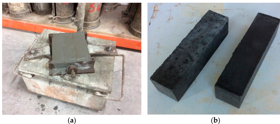
Figure 3. Mortar manufacture (a). Mortar specimens (b).
