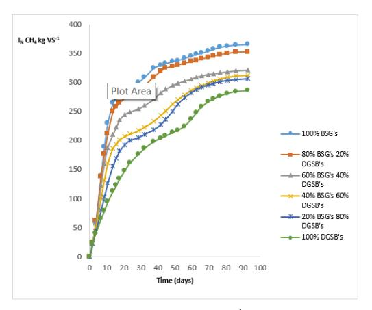
**Figure 1.** Total specific methane production in  $l_N CH_4 kgVS^{-1}$  from the BMP tests (SD for each sample: M1 (100% DGSBs), 12; M2 (80% DGSBs, 20% BSGs), 15; M3 (60% DGSBs, 40% BSGs), 19; M4 (40% DGSBs, 60% BSGs), 23; M5 (20% DGSBs, 80% BSGs), 15; M6 (100% BSGs), 22.
