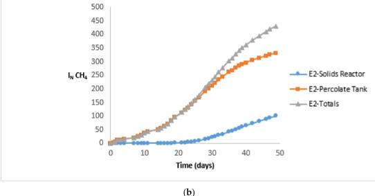
**Figure 2.** Methane production through time in  $l_N CH_4$  in experiments E1 (DGSBs as substrate, subfigure (**a**) and E2 (DGSBs as substrate with GAC used in the percolate tank, subfigure (**b**)) and the second phase of the experiment.
