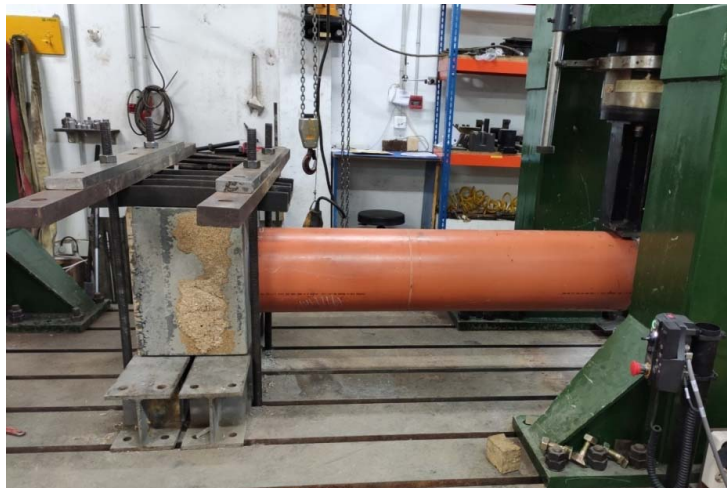
Fig. 4. Experimental setup of the tubular beams.
